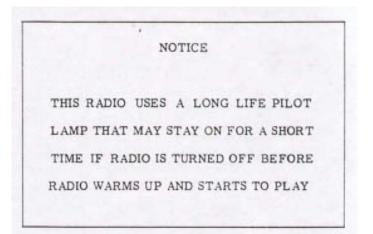
Figure 4. A notice attached to an AM-FM radio.
