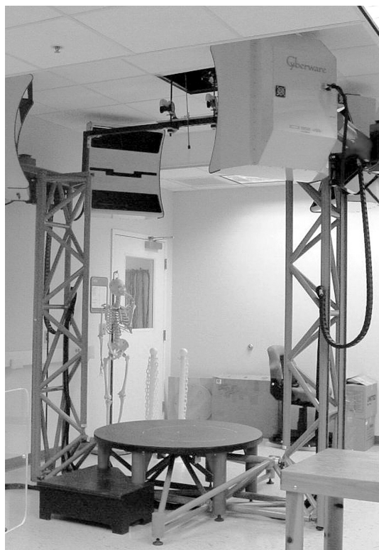
Figure 4. Equipment and positions used to evaluate the human-harness interface. (a) The custom-made suspension system (marked with a double circle) used in this study, and a standing posture with harness donned (A scan). (b) Suspended position (B scan). (c) Standing posture without harness (C scan). (d) The Cyberware WB4 3-D full-body scanner.
