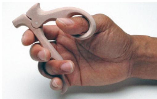
Figure 7. Design option showing the traditional grip style with contoured rings and pinky rest.
