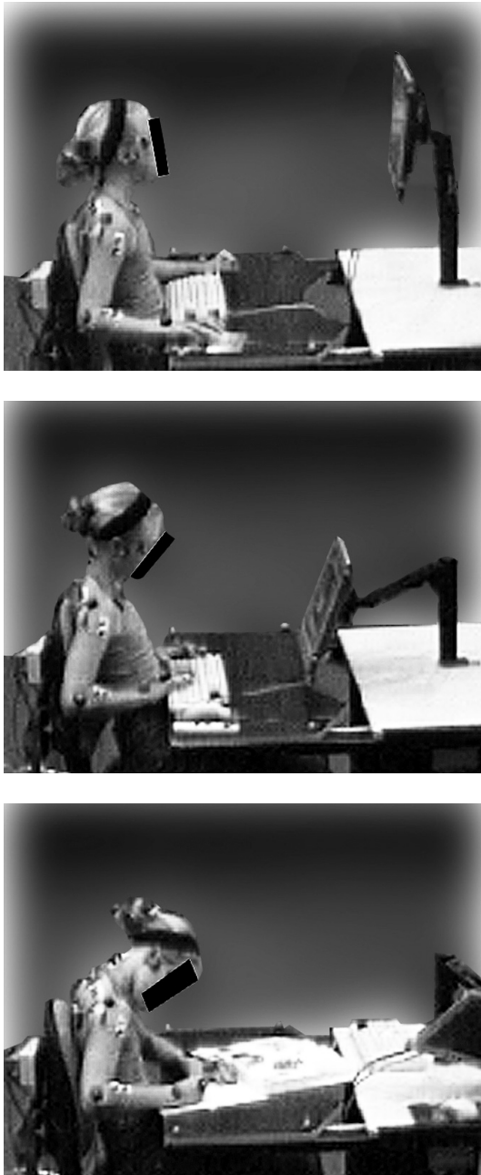
Figure 1. Workstation configurations for the high (top panel), mid (middle panel), and book (bottom panel) display conditions.
