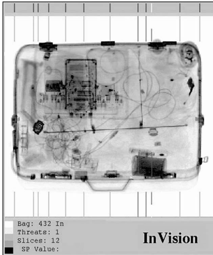
A can bomb is detected with the FAA-certified CTX 500 explosives detection system. AP Photo/InVision File. Used with permission.
