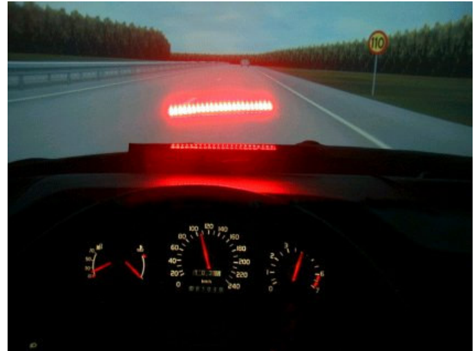
Figure 4. HUD warning reflected on the windshield
